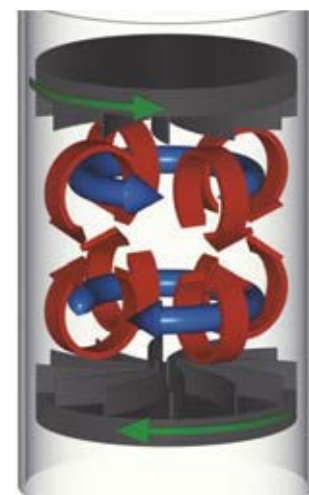
Figure 2. Diagram of the average flow between the two counter-rotating impellers. The toroidal flow is shown in blue and the poloidal pumping in red.
